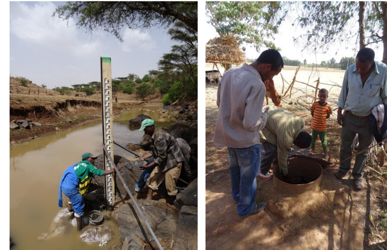
Reconstruction of the Kilti river gauge board (left) following damage during wet season floods and measuring depth to groundwater in a monitoring well
